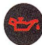
Engine Oil Pressure Warning Symbol
