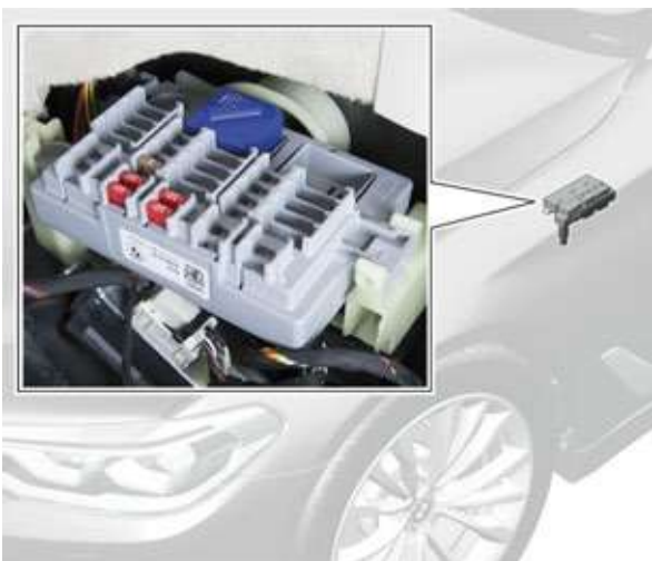
Power distribution box, front left
