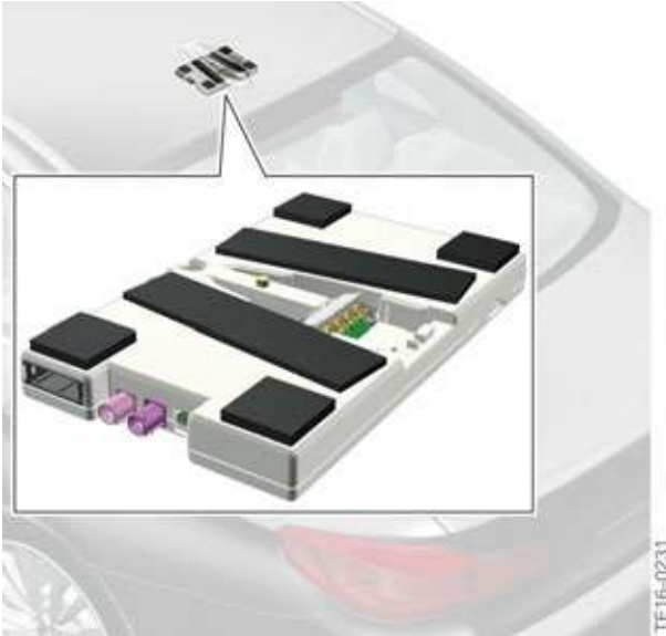
Telematic Communication Box (TCB)
