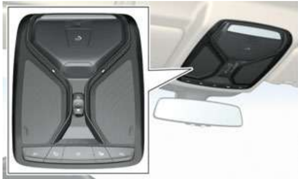
Roof function center (FZD)
