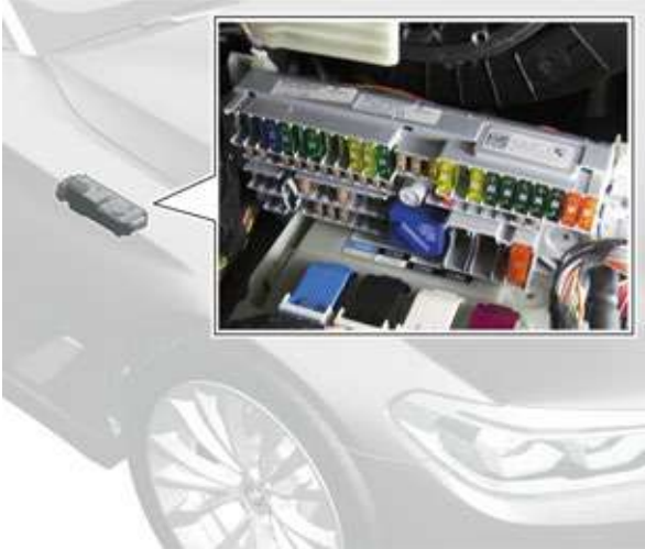
Power distribution box, front right
