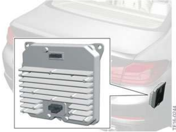
Power Control Unit (PCU)
