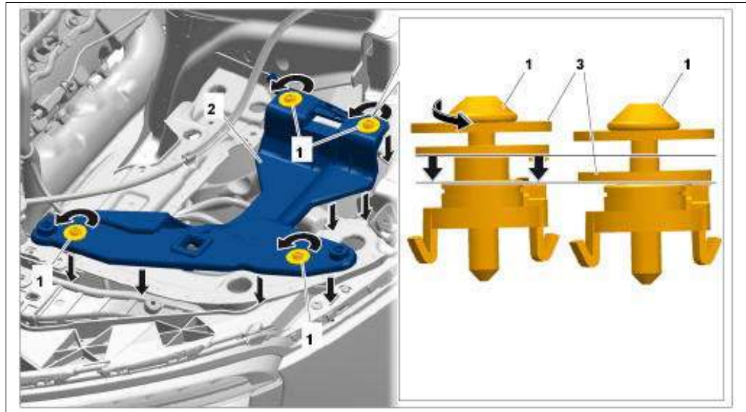
Fig 3: Identifying Lower Headlight Mounting
