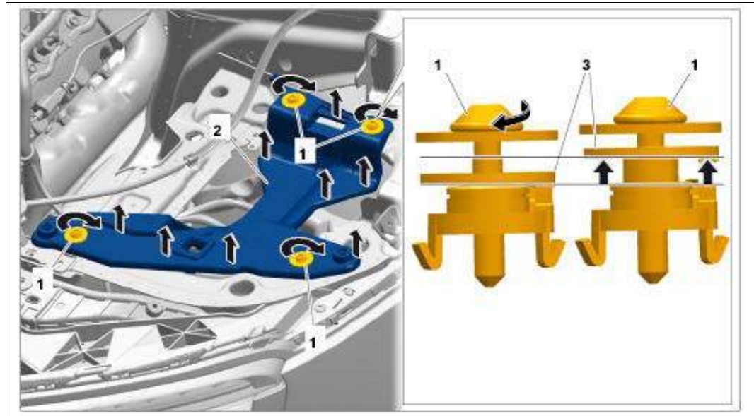
Fig 4: Raising Headlight Mounting
