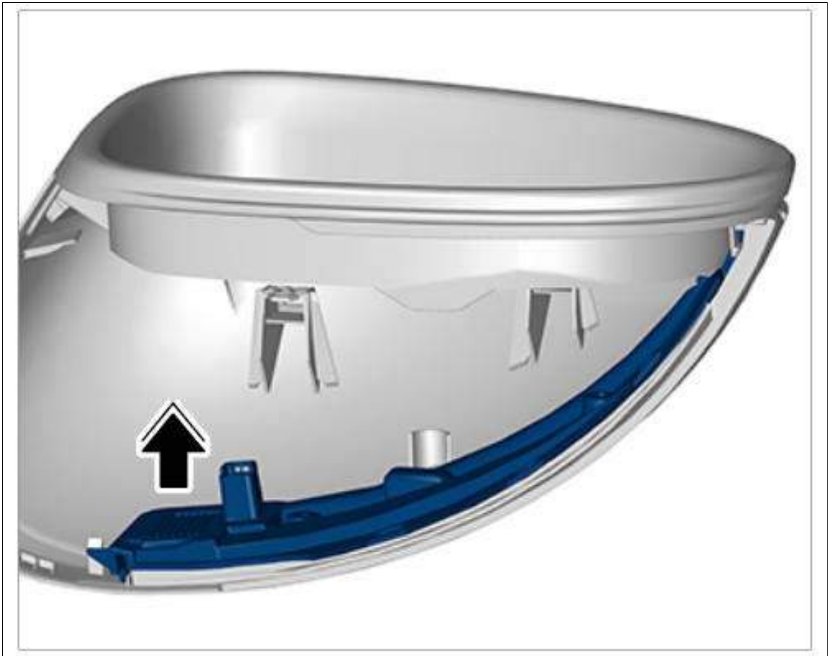
Fig 3: Removing Side Direction Indicator Light
