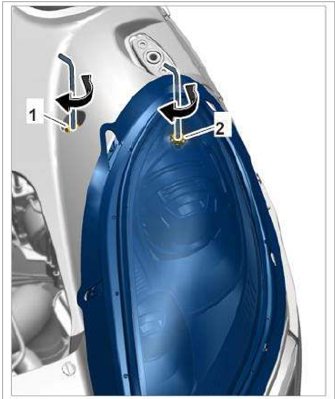
Fig 3: Turning Headlight Adjusting Screws
